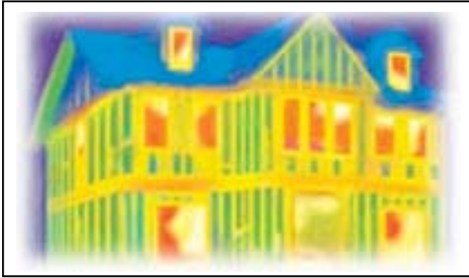
House with OSB and R-13 batts
