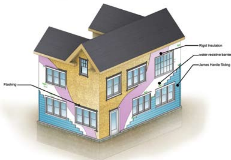
The house above shows how rigid foam insulation, HardieWrap® weather barrier and James Hardie® siding can eliminate air leakage and increase the whole wall R-value when properly installed, significantly decreasing energy costs.
